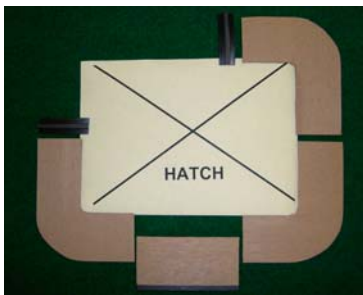
Fig 4 – Pre-cut Caulking and Infills
